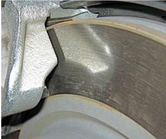
Brake friction material deposited on rotor.
