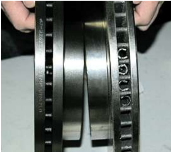
Light-weight rotor with thin plates.
