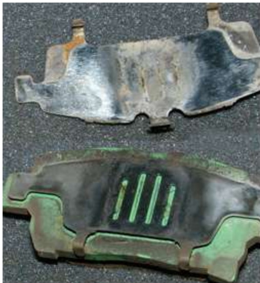
Two-piece brake pad shim from a Toyota Prius
