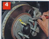
You know that this rotor has never been off because the factory-installed retaining clips are still on it. Remove them. It is not necessary to reinstall
