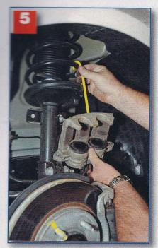
Use common sense and professional service procedures. Use a caliper hook to hang the caliper. Don't allow it to hang by the hose.
