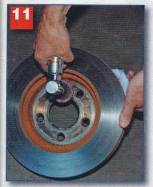
Also be sure to clean the inside surface of the rotor. Do this even when no rust or scale is present, as the rotor tends to build up a rust lip on the area just outside the lubricated area.
