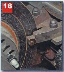
You can now run the bits in and make contact or perform a scratch cut. Back off the bits, run the bits the rest of the way in, set your depth of cut, engage the machine and do the cut.
