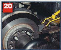
The lathe is about halfway out with the cut performed. This particular lathe can provide a proper finish with one cut, saving cost and time.
