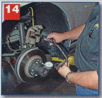
If you want to know the amount of rotor runout, put the adapter on, tighten the lug nuts and attach a dial indicator.
