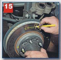
Mark the rotor, turn it a full revolution, note the amount of runout and write it on the rotor so you can remember it later on and note it on the work order. In this instance, there is 0.0025 inch, an amount usually just beyond specification but not yet causing pedal pulsation. However, if the situation continues, especially on one of these Mustangs that "go fast and stop hard," pedal pulsation may occur soon.
