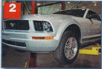
Vehicles such as the new-style Ford Mustang have a factory recommendation of on-car rotor turning to prevent pedal pulsation.
