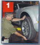
Before doing any brake work to solve pedal pulsation, grasp the wheel and tire as shown and check for inand-out movement. If there is a loose wheel
