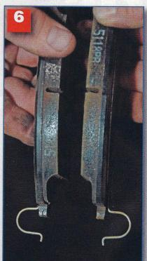
Check the pads for tapered wear, unusual sharp edges and more wear on one pad than the other, an indication of a slide problem. Don't just remove and discard them. Look at them to see what is going on.
