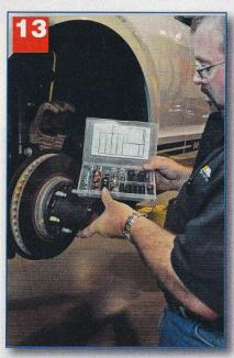
Certain OE lug nuts, like those on this Mustang, do not allow the adapter to be installed because of their larger diameter. This lathe includes a set of lug nuts with a smaller outside diameter that enable the adapter to be easily installed.
