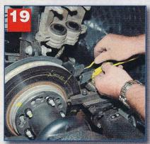
Before you actually take the cut, put a silencer on the rotor. Although not always necessary, using a silencer will prevent an irritating, high-pitched sound and possible chatter that can result in an irregular surface. It's just a smart service procedure.
