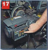
Press the button for automatic runout compensation. This takes only a few seconds, and when it's finished the "ready" sign will come on.
