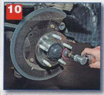
If there is any buildup use a Scotch-Brite type of cleaning pad or a special tool that fits over the stud to remove it. Rust and scale buildup in this area causes rust jacking that in turn causes a large amount of runout at the edge of the rotor.
