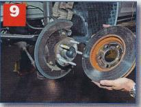
Lift the rotor from the hub and look at the back side. Ford commonly lubricates the contact area between the rotor and the hub. That was the case on this vehicle and there is no significant rust and scale buildup.
