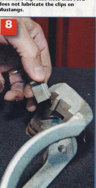
The coating on the back side of the clip is not allowing any rust or scale to build up, but the front side – where the raw steel pad contacts it – does have a buildup that can limit the pad's sliding action.
