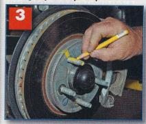
Ford Motor Co. match-mounts rotors to hub faces. Mark the rotor, mark the stud and be sure to install the rotor at the same location to avoid causing a problem that was not there before.
